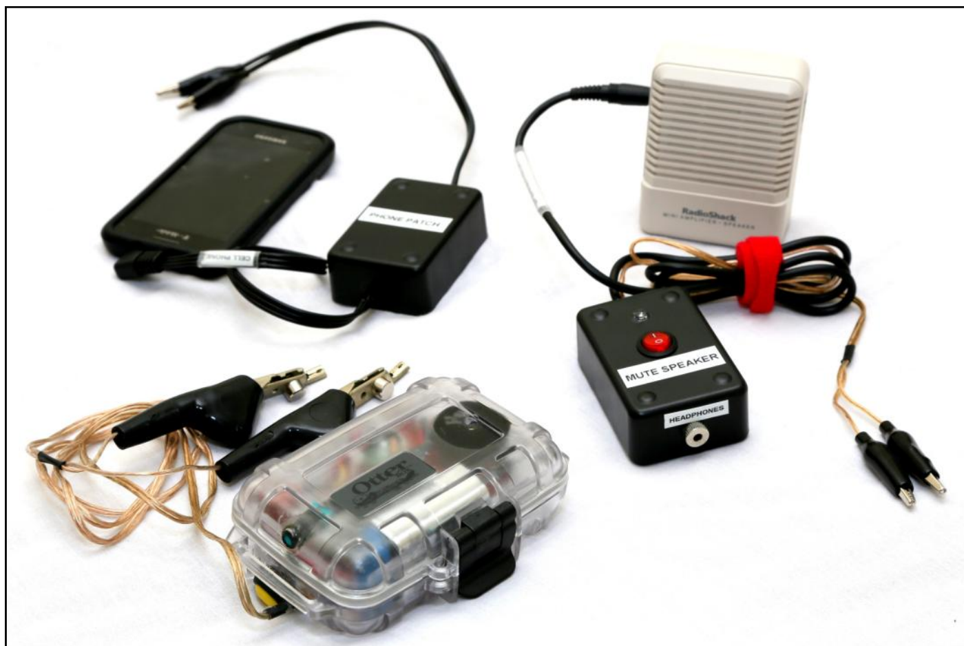
(Clockwise from bottom left) Pocket Field Telephone, Smartphone Patch, and Speaker Interface
