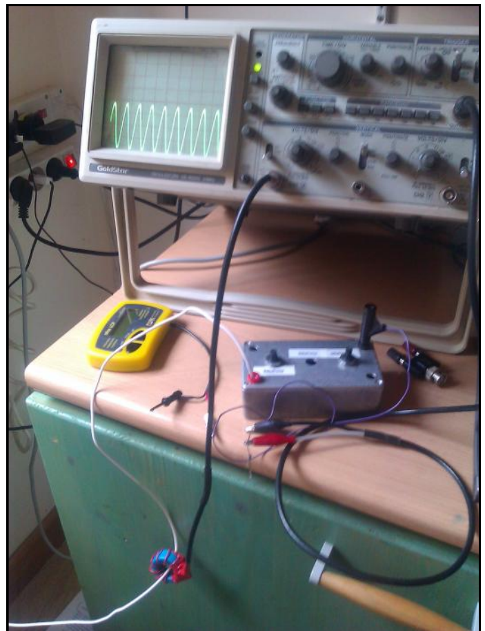
Signal generator connected to antenna wire through adjustable inductor box to determine resistive ground impedance (current maximum measured by Rogowski coil).
