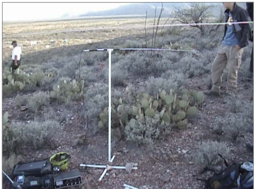
Surface setup with the small portable antenna. The full wave loop was also used on this hill.
