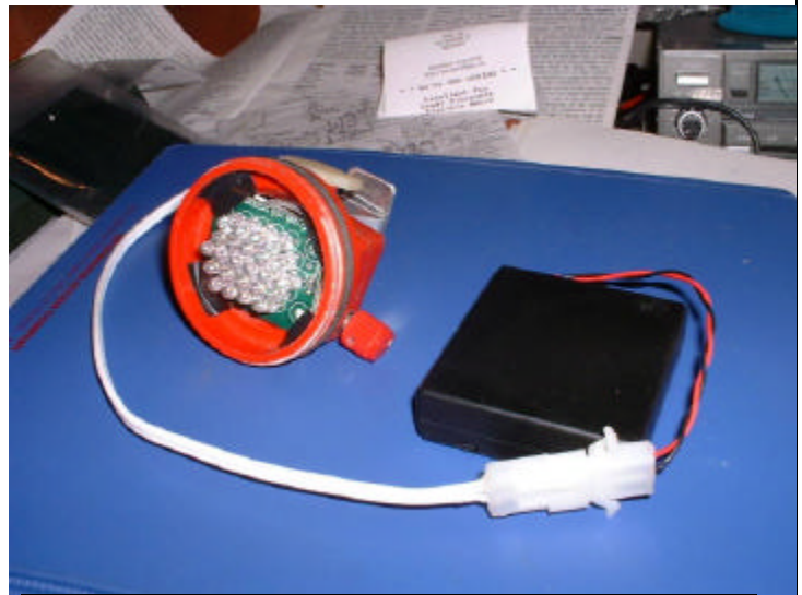
Battery Pack with LED s in place
